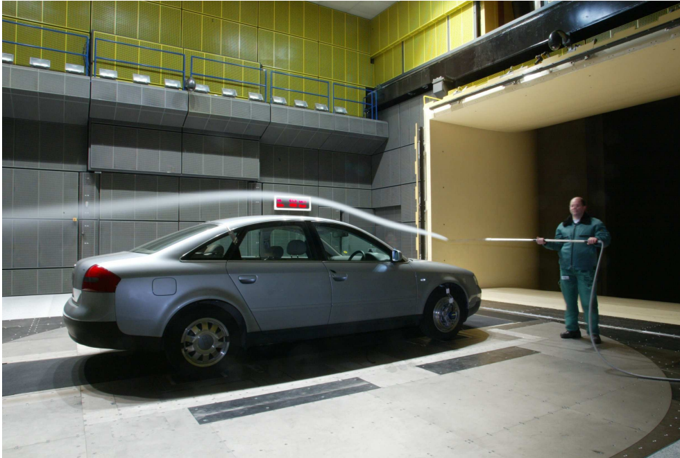
Figure 1.5: Measuring the aeroacoustics in a wind tunnel [5].
